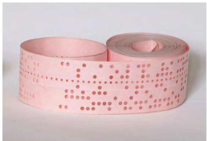
Eight-hole punched paper tape example
